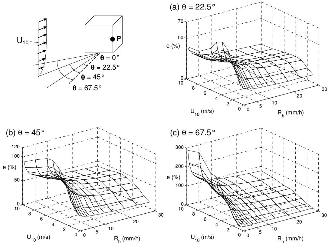
Fig. 6. A graphical presentation of the errors (percentages) that are introduced by the use of the cosine projection at position P of the windward facade. The errors are given as a function of  $U_{10}$  and  $R_h$  for the three wind directions.
