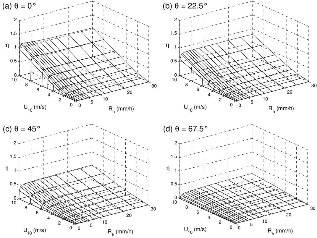
Fig. 3. CFD-simulation results: catch-ratio charts for position P on the windward facade of the cubic building model and for four different wind directions. Each catch-ratio chart displays the catch ratio  $\eta$  as a function of the reference wind speed  $U_{10}$  and the horizontal rainfall intensity  $R_h$  for a fixed wind direction.
