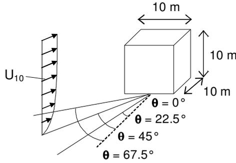
Fig. 1. Low-rise cubic building model ( $l \times b \times h = 10 \times 10 \times 10 \text{ m}^3$ ). CFD simulations are conducted for four different wind directions.
