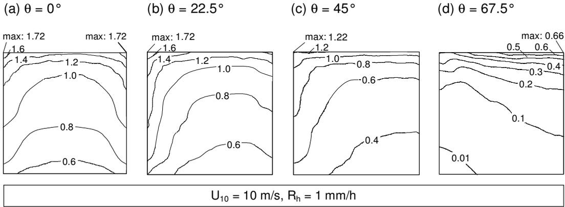
Fig. 2. CFD-simulation results: contours of the catch ratio  $\eta$  on the windward facade of the low-rise cubic building model for  $U_{10} = 10$  m/s,  $R_h = 1$  mm/h and for four different wind directions.
