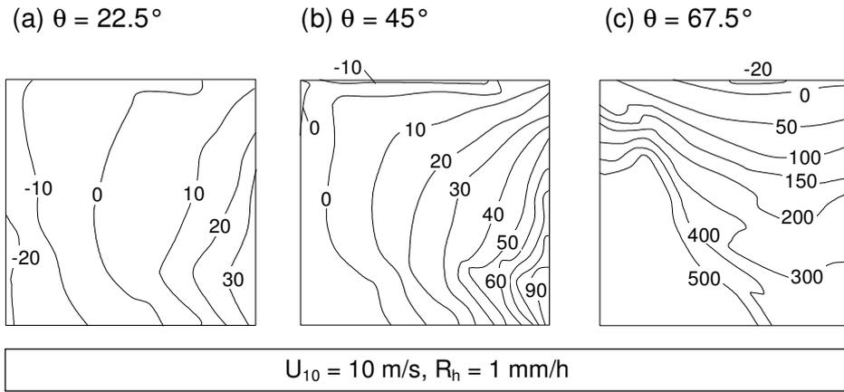
Fig. 5. A graphical presentation of the errors (in percentages) that are introduced by the use of the cosine projection for  $U_{10} = 10$  m/s,  $R_h = 1$  mm/h and for the three wind directions.
