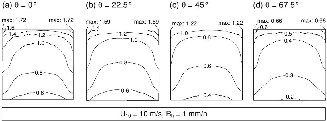
Fig. 4. Results of applying the cosine projection to the CFD result in Fig. 2a. All figures are for  $U_{10} = 10$  m/s and for  $R_h = 1$  mm/h.
