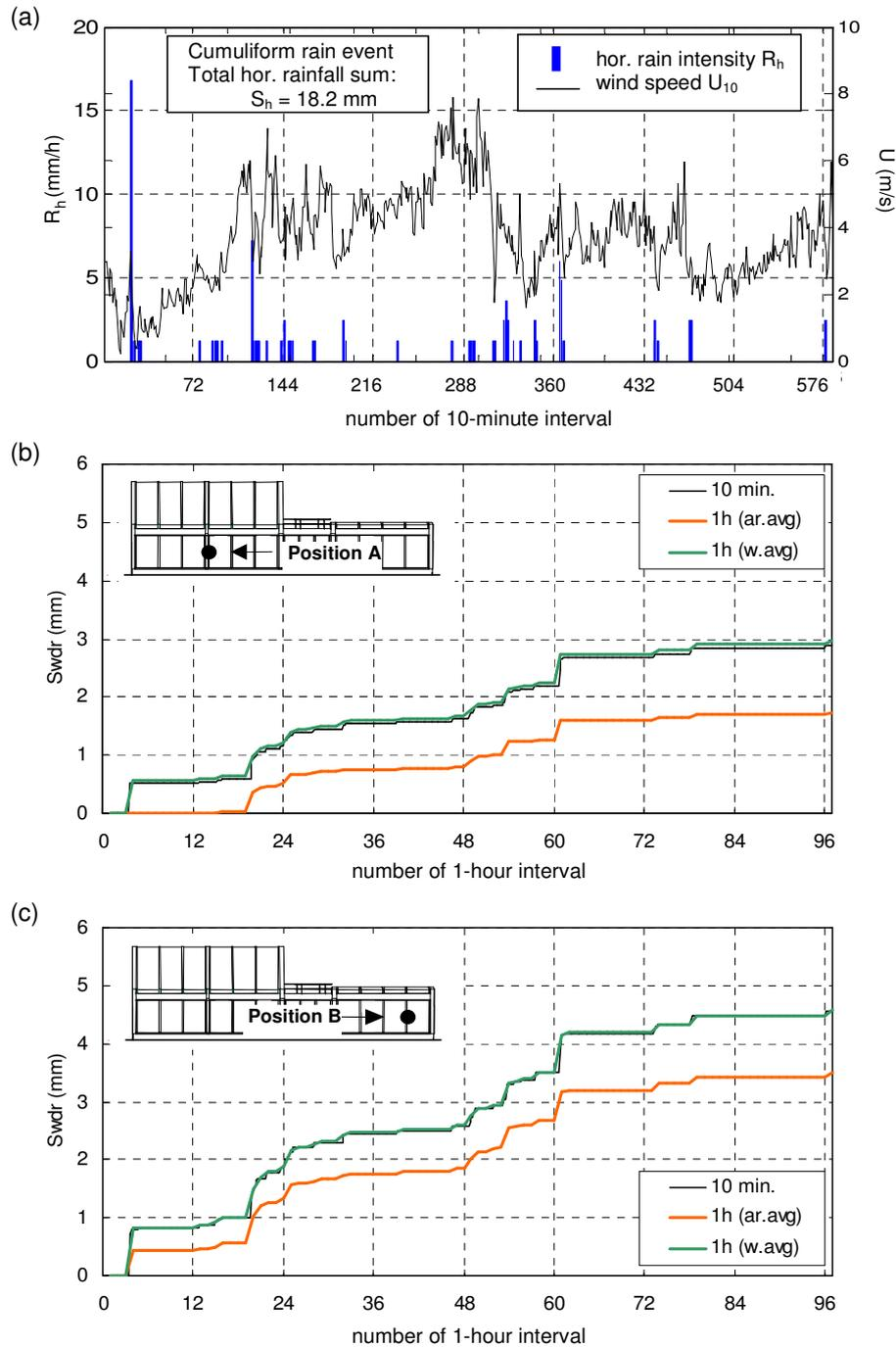
Fig. 7 (a) Cumuliform rain event: 10-minute data of the reference wind speed  $U_{10}$  and the horizontal rainfall intensity  $R_h$ . (b-c) Cumulative wind-driven rain  $S_{wdr}$  calculated with the catch-ratio charts generated by the CFD model at (b) position A and (c) position B of the VLIET building.  $S_{wdr}$  is calculated in three different ways: (1) using 10-minute data of  $U_{10}$  and  $R_h$ ; (2) using arithmetically-averaged hourly data; (3) using weighted-averaged hourly data.
