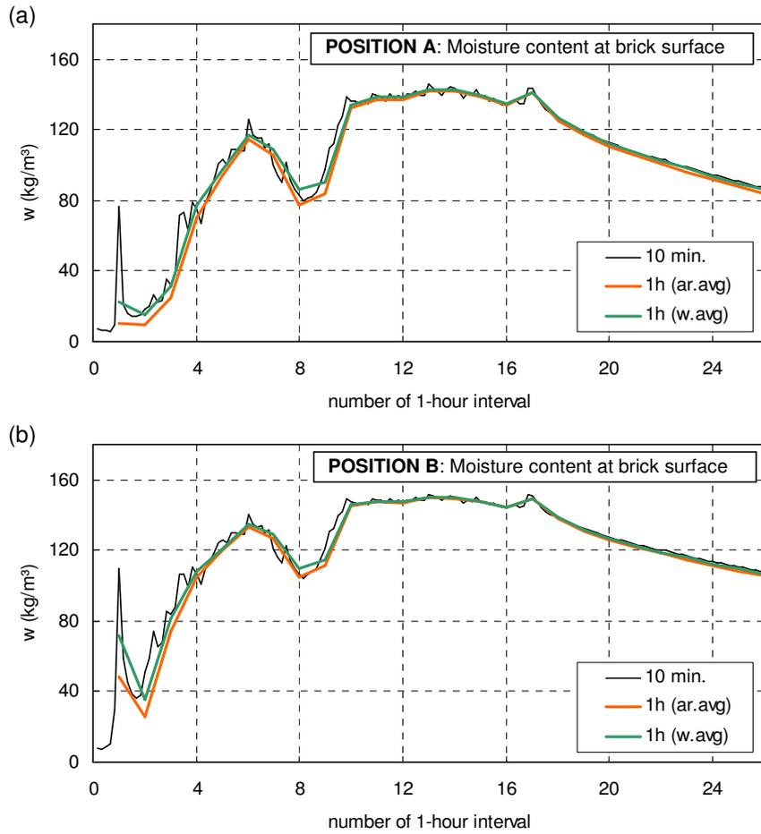
Fig. 11. Calculated moisture content at the outer surface of the brick wall during the rain event given in Fig. 10a for (a) position A and (b) position B of the VLIET building. The results have been calculated with three different sets of wind-driven rain data (see Fig. 10b-c).
