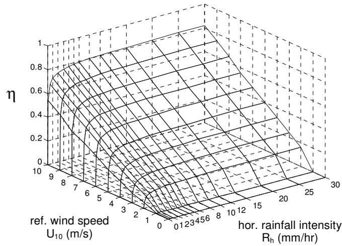
Fig. 1. Typical example of a catch-ratio chart or  $\eta$ -chart that presents the catch ratio  $\eta$  as a function of the reference wind speed  $U_{10}$  and the horizontal rainfall intensity  $R_h$ , for a given position on the building facade and for a given wind direction. Data points are provided for a discrete set of couples  $(U_{10}, R_h)$ . Intermediate values are obtained by linear interpolation (Blocken and Carmeliet, 2002).
