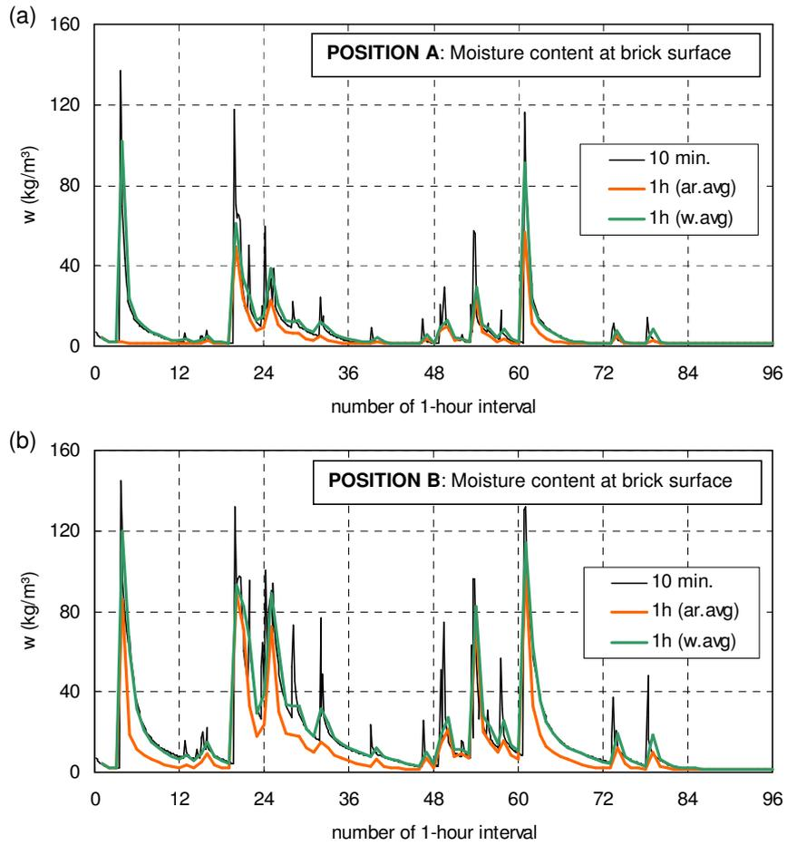
Fig. 8 Calculated moisture content at the outer surface of the brick wall during the rain event given in Fig. 7a for (a) position A and (b) position B of the VLIET building. The results have been calculated with three different sets of wind-driven rain data (see Fig. 7b-c).
