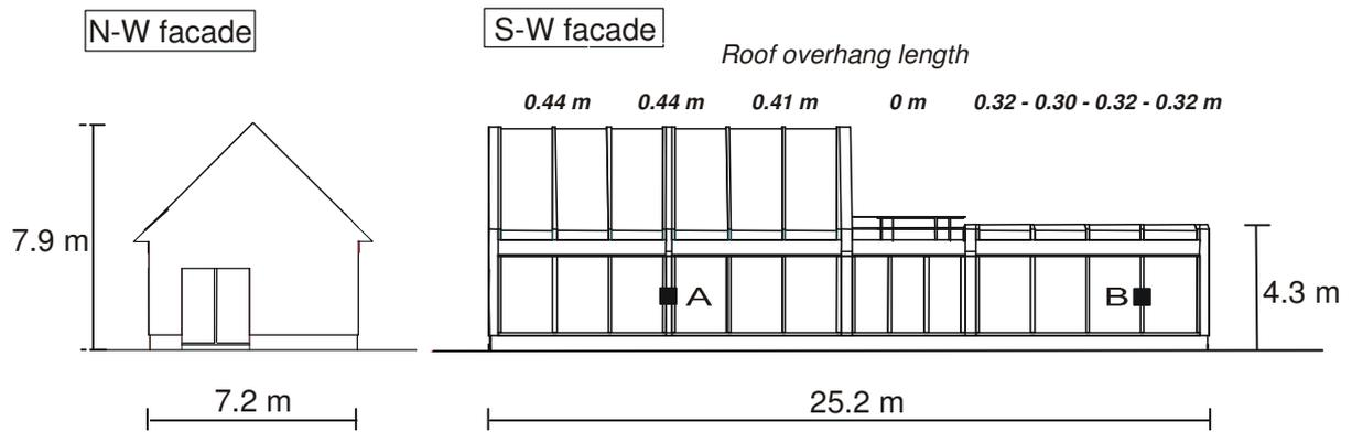
Fig. 3. North-west and south-west facade of the VLIET test building. The building dimensions including roof overhang length are given. The positions A and B on the facade that will be used in the present paper are indicated.
