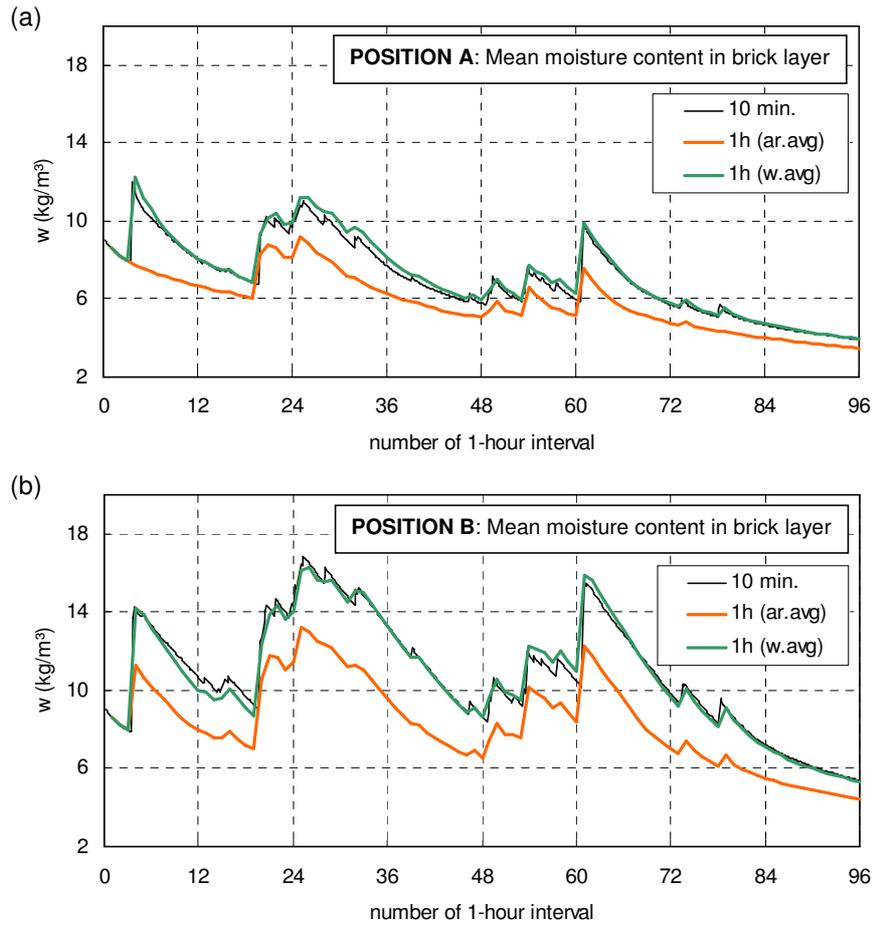
Fig. 9 Calculated mean moisture content in the brick layer during the rain event given in Fig. 7a for (a) position A and (b) position B of the VLIET building. The results have been calculated with three different sets of wind-driven rain data (see Fig. 7b-c).
