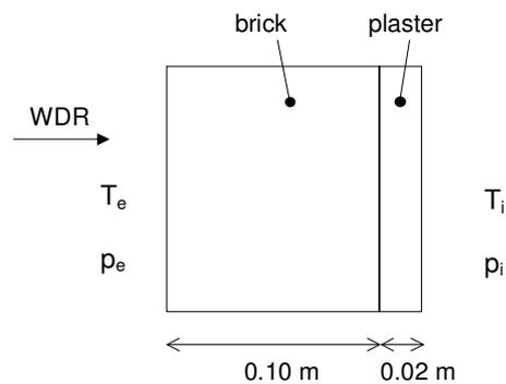
Fig. 4. Configuration of the 1D wall model used for the heat and moisture transfer simulations. Indication of the variables representing the boundary conditions ( $T$  = temperature,  $p$  = vapour pressure,  $e$  = exterior,  $i$  = interior).
