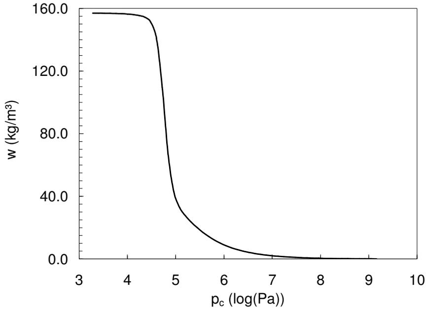
Fig. 5. Moisture retention curve for the ceramic brick.
