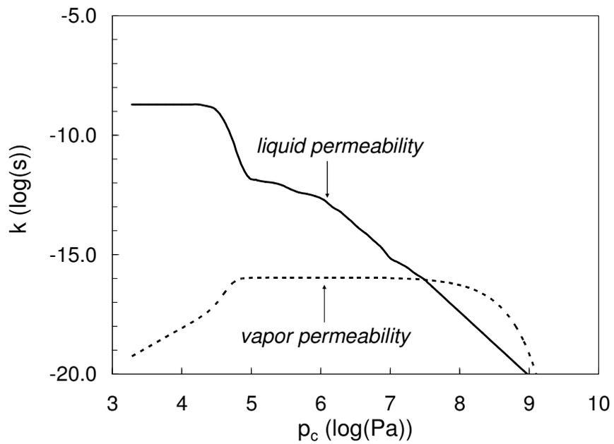
Fig. 6. Moisture (liquid and vapour) permeability as a function of the capillary pressure for the ceramic brick.
