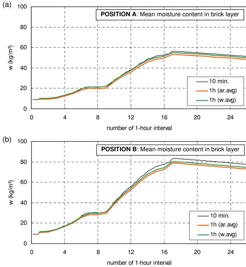
Fig. 12 Calculated mean moisture content in the brick layer during the rain event given in Fig. 10a for (a) position A and (b) position B of the VLIET building. The results have been calculated with three different sets of wind-driven rain data (see Fig. 10b-c).
