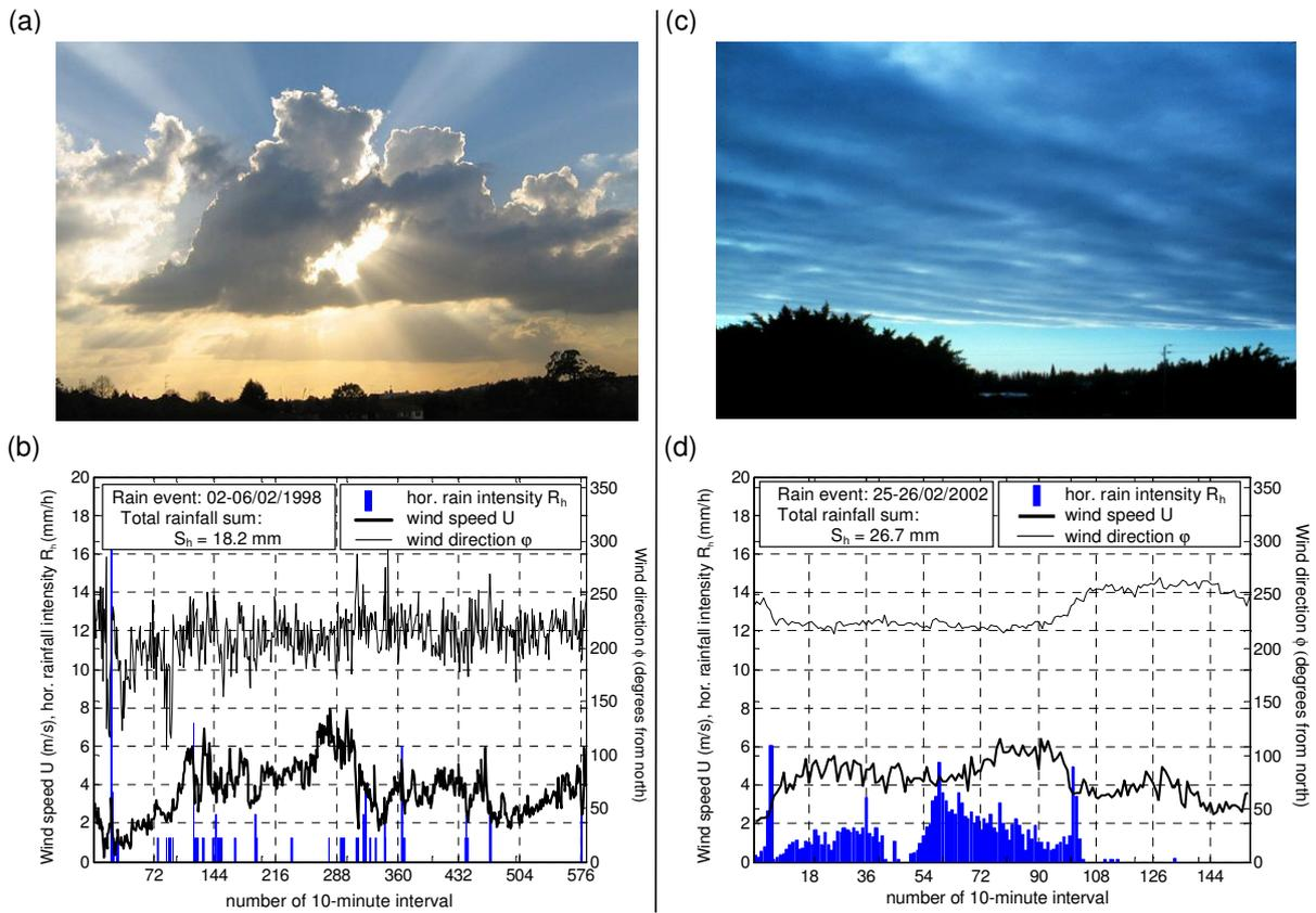
Fig. 2. Typical images of cumuliform clouds and stratiform clouds and the resulting rainfall records: (a) Cumuliform cloud; (b) Cumuliform rain event; (c) Stratiform cloud; (d) Stratiform rain event. The measurements were made at the VLIET test site (Blocken and Carmeliet, 2005).
